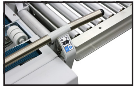
Quick size change with top wheel and tilting guide rails
